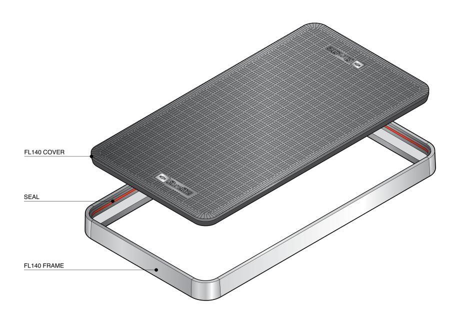
55" x 28" flat sealed composite cover with an aluminum frame.
