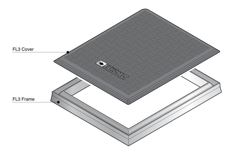
30" x 24" raised composite cover with an aluminum frame.
