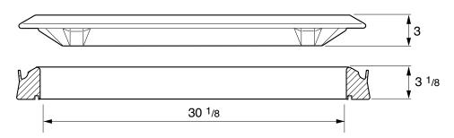
30" x 24" raised composite cover with an aluminum frame.
