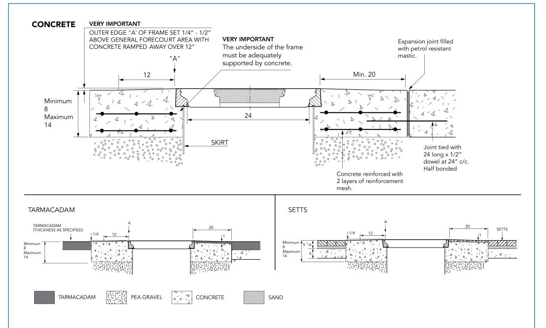
24" diameter flat sealed composite cover with a central port cover and composite frame.
